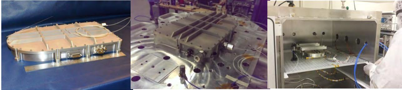
Figure 1. A 20 W fiber amplifier laser optical module (LOM) for lidar and optical communications (left), on a vibration table (center), and in a thermal vacuum chamber (right).
