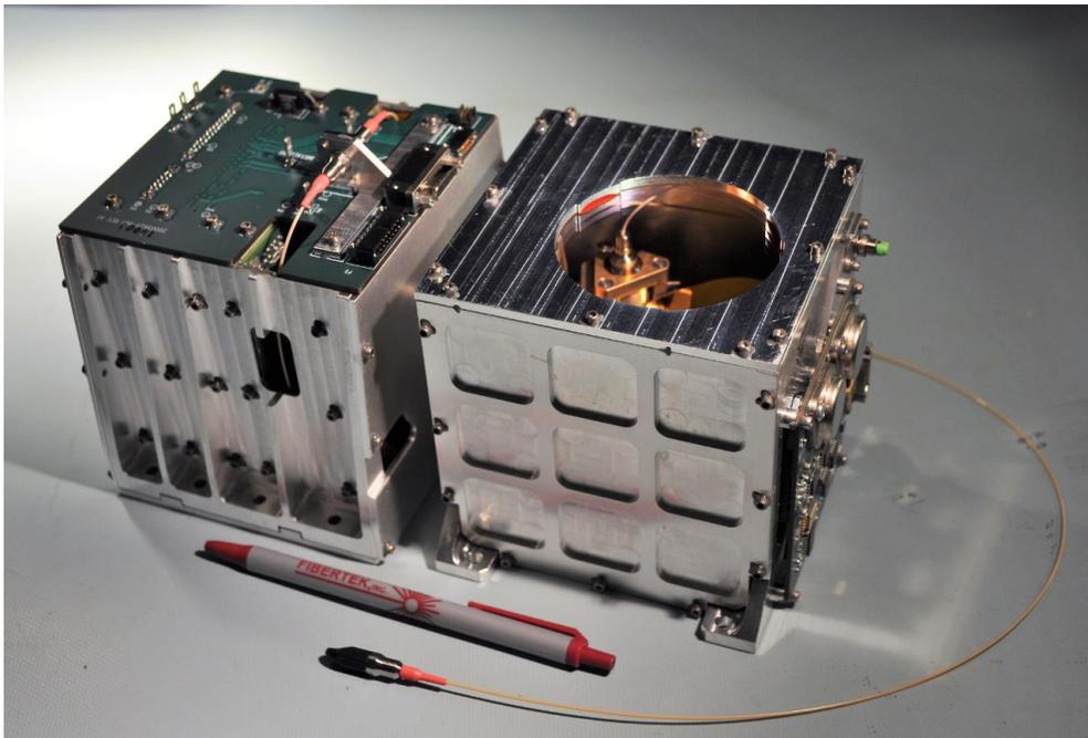
**Figure 3: 1x2U CubeSat lasercom terminal consisting of (left) electronics module and (right) optical module**
