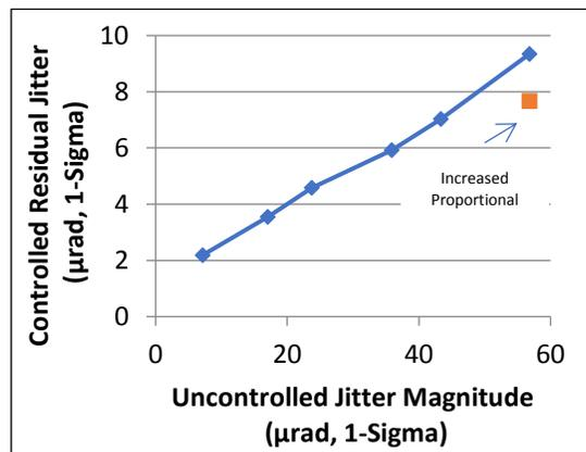
**Figure 4: On-Orbit Fine-Steering Jitter Mitigation, Residual Jitter vs. Uncontrolled Jitter**
