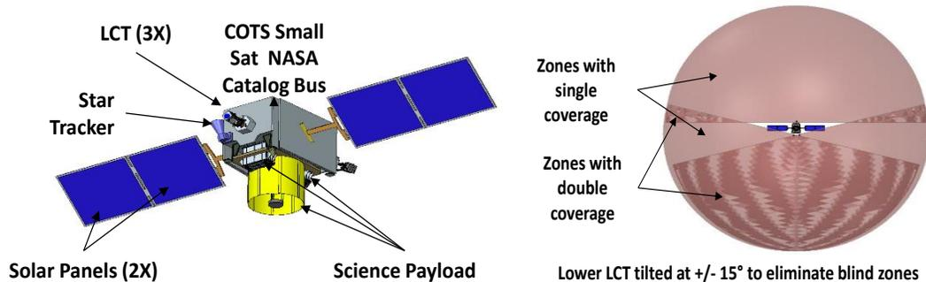
**Figure 2: (Left) Example of a SmallSat with a science payload and multiple LCT's for crosslink and downlink and (Right) zones of coverage with 3 LCT's.**
