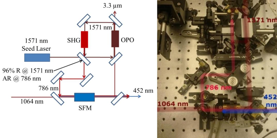
Figure 7: Schematic and photograph of the nonlinear conversion set-up
