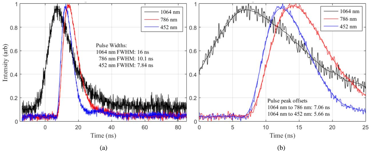
Figure 10: a) temporal overlap of the pump (1064 nm), red (786 nm), and blue (452 nm) pulses, and b) inset
