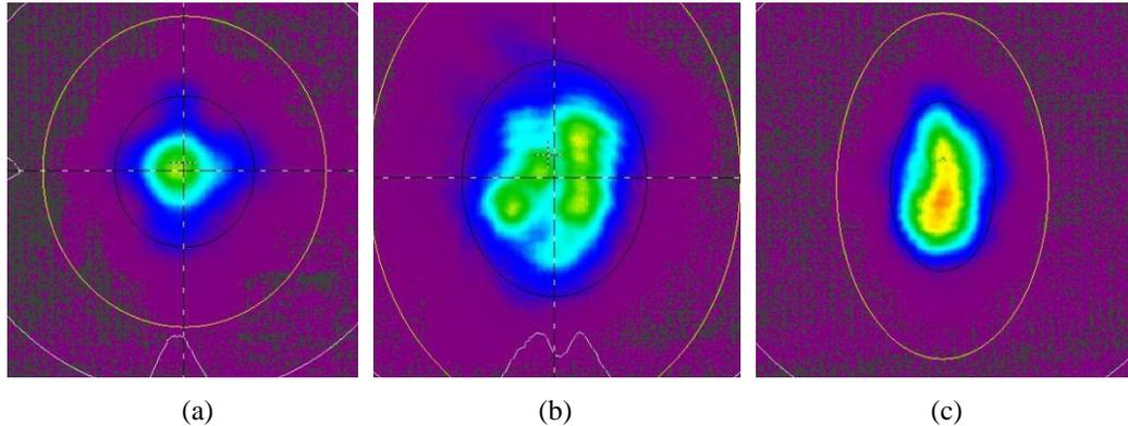
Figure 9: Beam profiles at SFM crystal a) 1064 nm, b) 786 nm, and c) 452 nm
