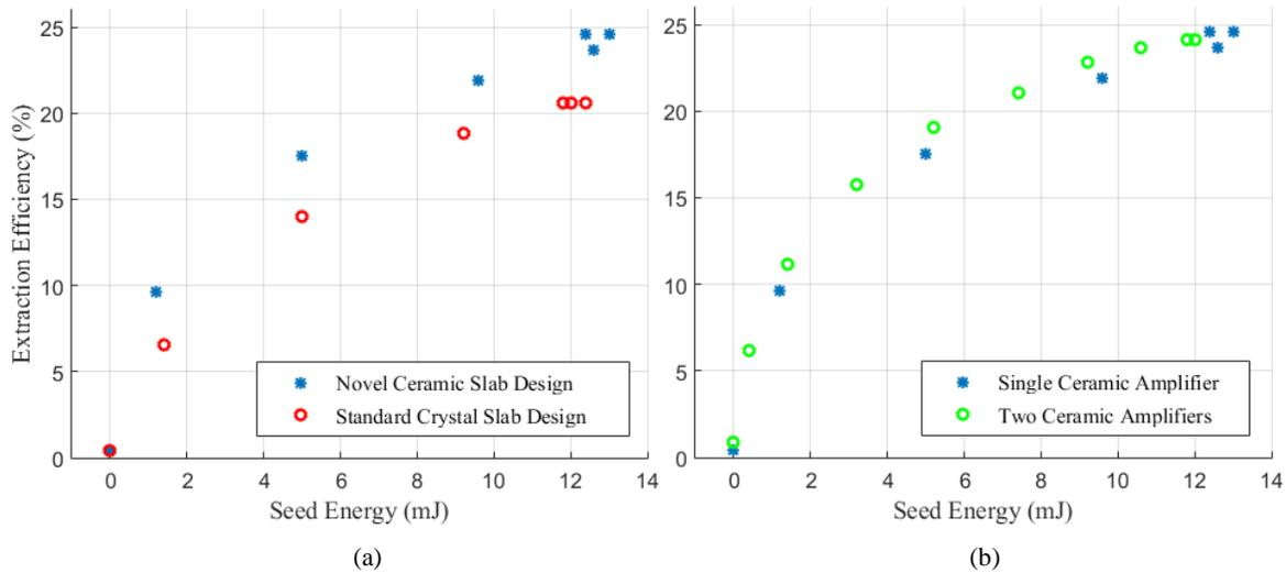
Figure 4: a) comparison of extraction efficiency of a single standard slab vs. a novel slab; the novel design shows a 19% increase over previous designs, b) comparison of extraction behavior of one vs. two novel amplifier stages shows consistent performance
