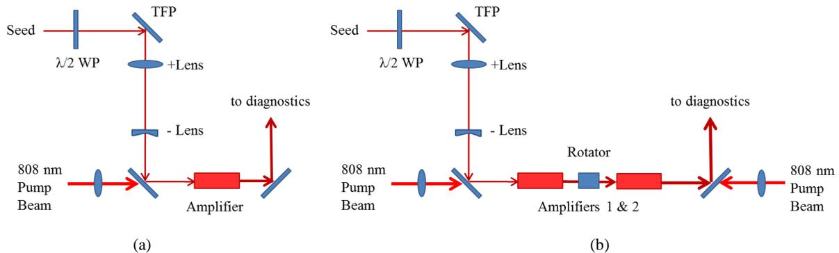
Figure 3: Schematic of amplifier testing set ups: (a) single amplifier testing set up is used to compare the performance of a single slab of each the standard and novel designs, and (b) two amplifiers of the novel design.
