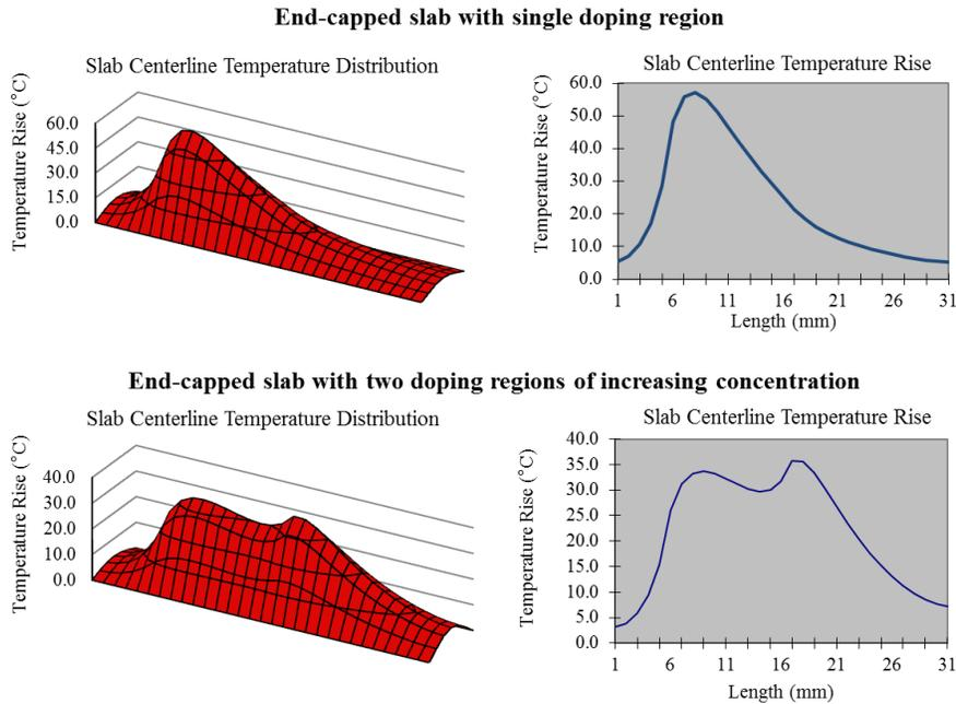
Figure 2: Calculated thermal profiles for single layer slab and multi-layer rods
