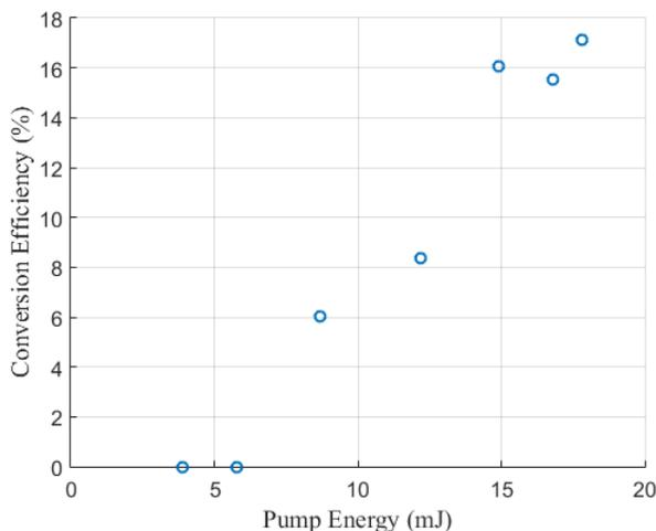
Figure 8: Conversion efficiency shown as a function of applied pump energy, and the maximum conversion efficiency from 1064 nm to 452 nm was 17.1%.
