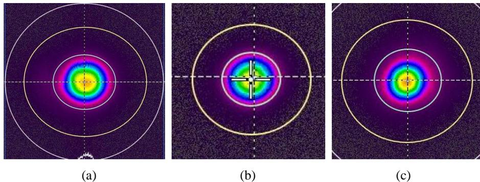
Figure 5: Far field beam images of a) a single stage of new amplifier design, b) a single stage of the standard amplifier design, and c) two stages of the new amplifier design.
