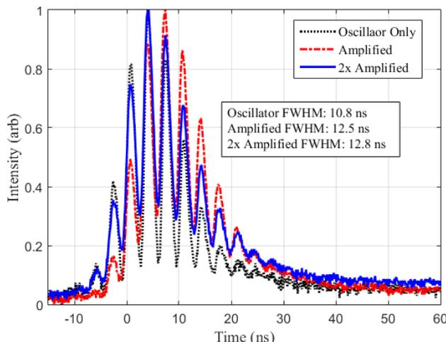
Figure 6: Temporal pulse width increases with amplification from 10.8 ns to 12.8 ns
