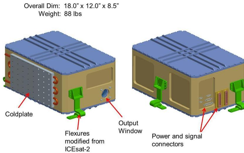
Figure 6. Dimensions, weights and interfaces of the UVLD laser optics module
