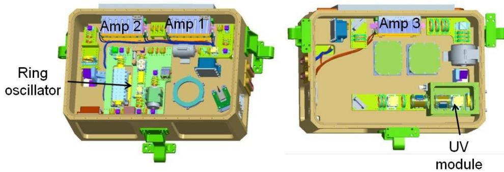
Figure 5. Overview of the two optical compartments in the UV Lifetime Demonstrator
