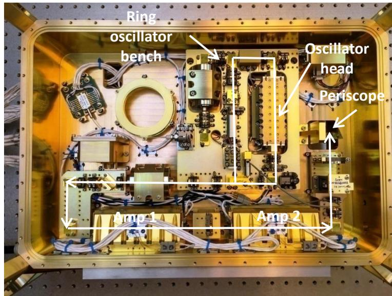
Figure 7. View of compartment containing the ring oscillator, amplifier 1, and amplifier 2
