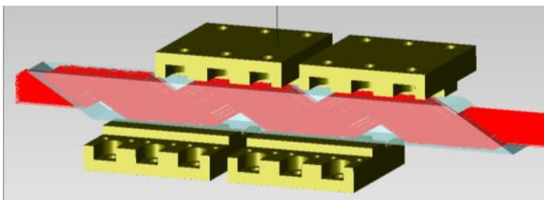
Figure 4. Schematic of the pump diode configuration for the power amplifier pump design. Four diode stacks are centered on the central four bounce points of a six-bounce zig-zag slab.
