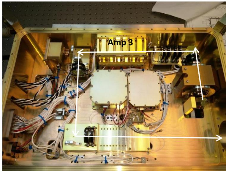
Figure 8. View of compartment containing amplifier 3. The nonlinear converters are not yet installed.
